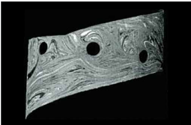
Figure 8: Photograph of the Unwrapped Channel Round Pin Mixing Section Showing Poor Distributive Mixing
