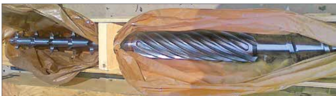
Figure 9: Brand New Screw Showing Dispersive and Distributive Mixing Sections
