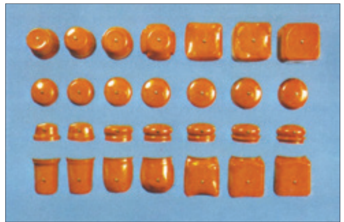
Figure 59: Blowing Investigation (coffee container with lid)
