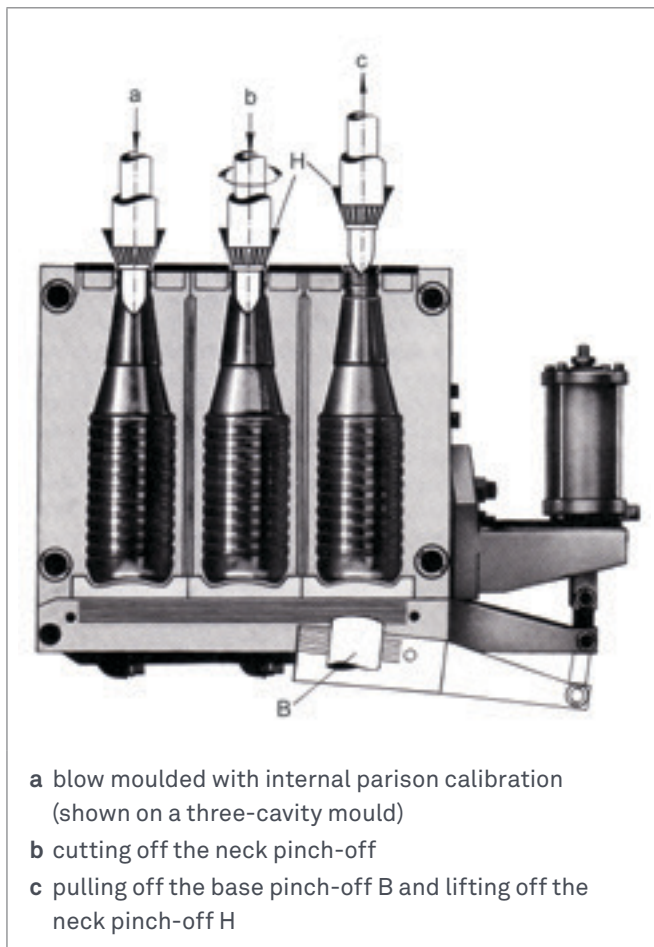
Figure 40: Automatic Separation of Neck and Base Pinch-off from a Bottle
