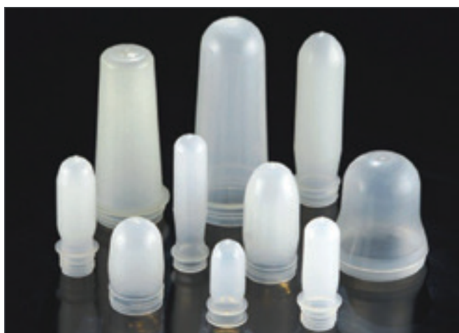
Figure 49b: Collection of Injection Moulded "Pre-forms" Awaiting Blow Moulding into Containers
