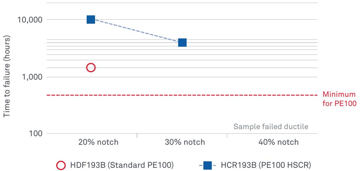
NOTE: Test covered 110mm pipes with varied notch depth tested in hydrostatic pressure test at 920kPa/80°C
