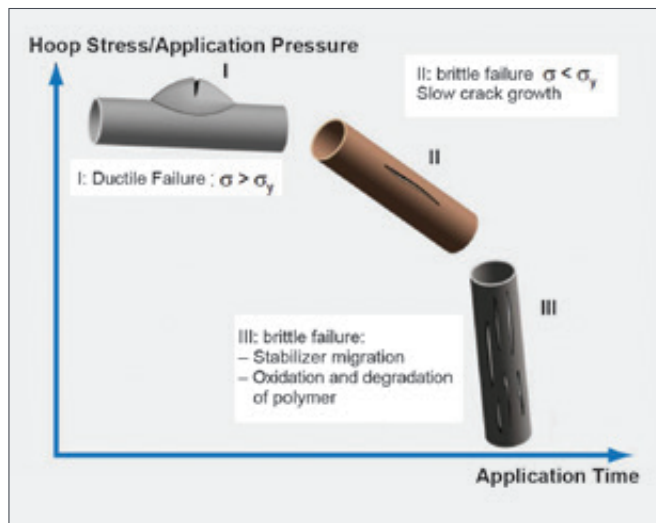
Figure 23: Representation of Pipe Curve According to the 3-stage Model (Illustration by Studsvik Material AB now known as Exova)
