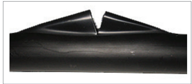
Figure 24: Pipe Failed in Ductile Mode
