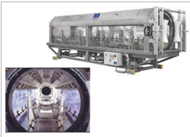
Figure 12: Photographs of Spray Water Bath
