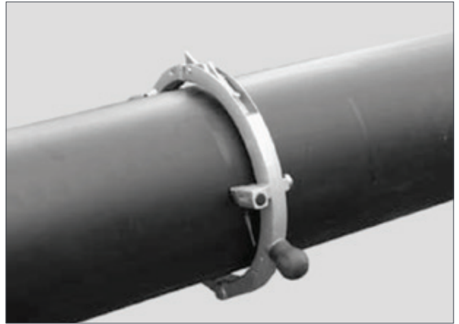
Figure 47: Installation of Detachable Rotary Peeler to Service Pipe
