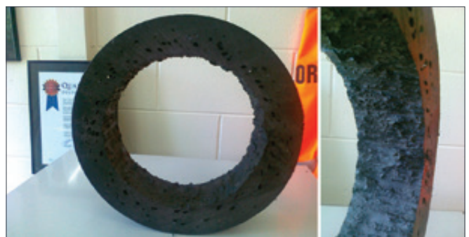
Figure 2: Photograph illustrating a Pipe with Voids and a Rough Pipe Surface due to Excessive Moisture in the Polymer Compound
