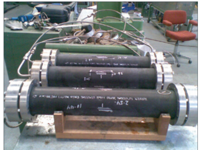
Figure 29: Pipes Notched and Assembled to be Tested for Slow Crack Growth Property as per ISO 13479. Pipes made from Qenos Pipe Grade Alkadyne HDF193B.
