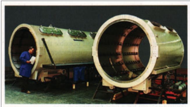
Figure 11: Vacuum Tanks for Sizing Pipes up to 1,400 mm in Diameter
