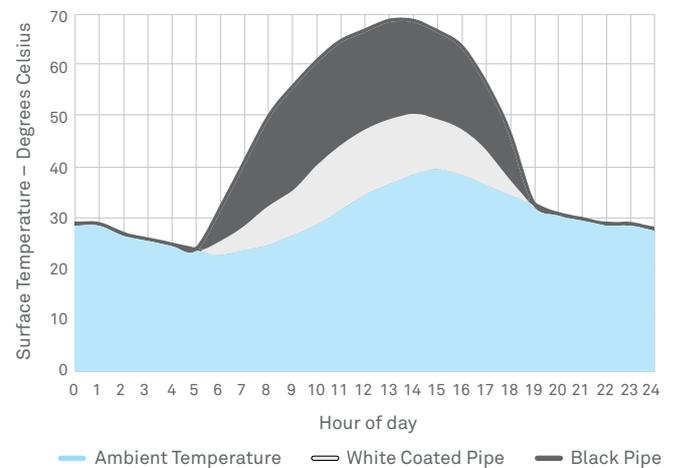
**Figure 2. Typical thermal effects of solar radiation on white coated pipe and black pipe over 24 hours**
