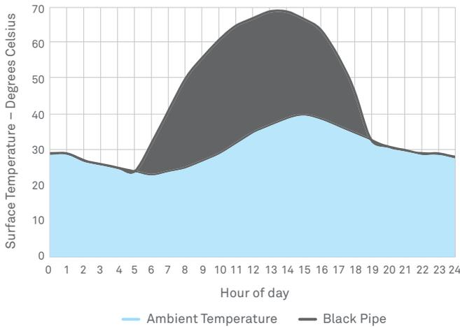
**Figure 1. Typical thermal effects of solar radiation on black pipe over 24 hours**
