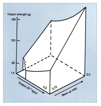
**Figure 4**: Variation of Impact Strength with Blow-up Ratio and Output Rate of an *Alkathene* LDPE Grade of MFI 2.0 and Density 0.921 g/cm3 (Film Thickness 38 micron)
