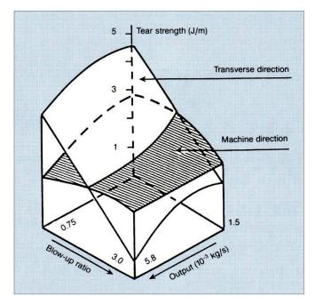
Figure 2: Variation of Tear Strength with Blow-up Ratio and Output Rate of an *Alkathene* LDPE Grade of MFI 2.0 and Density 0.921 g/cm3 (Film Thickness 38 micron)
