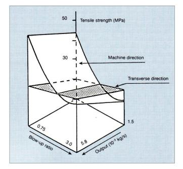
Figure 1: Variation of Tensile Strength with Blow-up Ratio and Output Rate of an *Alkathene* LDPE Grade of MFI 2.0 and Density 0.921 g/cm<sup>3</sup> (Film Thickness 38 micron)
