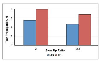
Figure 3: Effect of Blow-up Ratio on Tear Propagation for Alkamax mLLDPE Grade of MFI 1.0, Density 0.918 g/cm3 (Film Thickness 25 micron)
