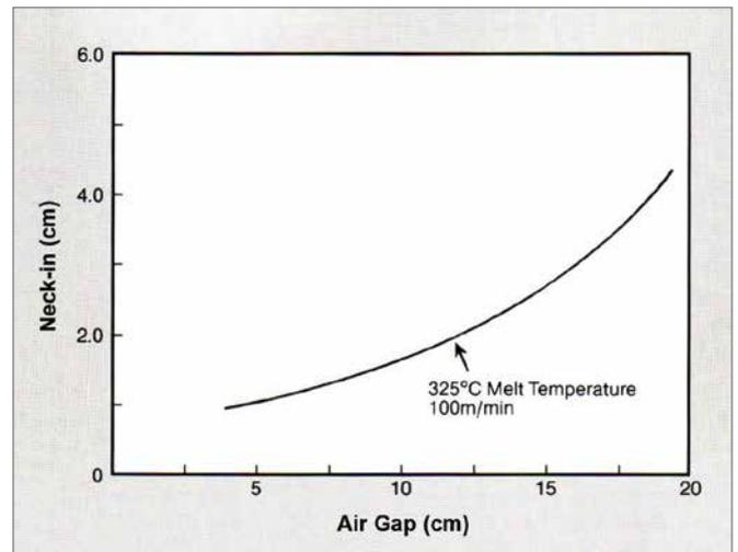
**Figure 8:** Typical Effect of Air Gap Distance on Neck-in
