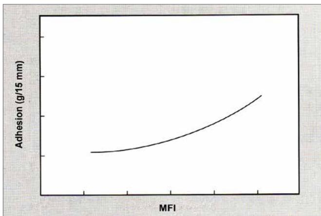
**Figure 10:** Effect of MFI on Adhesion of Extrusion-Coated LDPE to Porous Substrates
