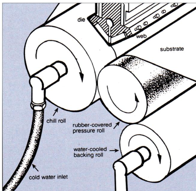
**Figure 3:** Typical Extrusion Coating Nip Roll Assembly
