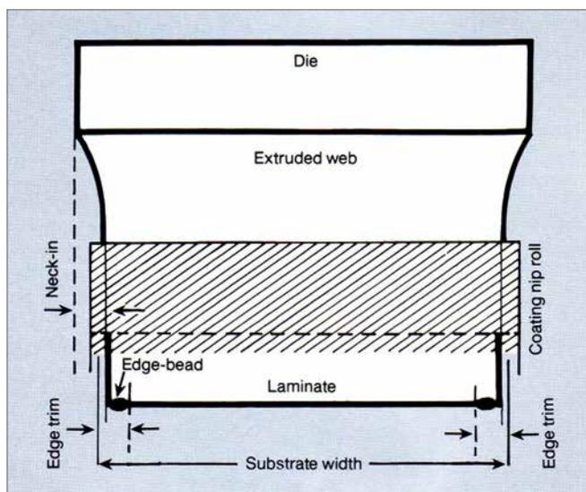
**Figure 4: “Neck-in” During Extrusion Coating**
