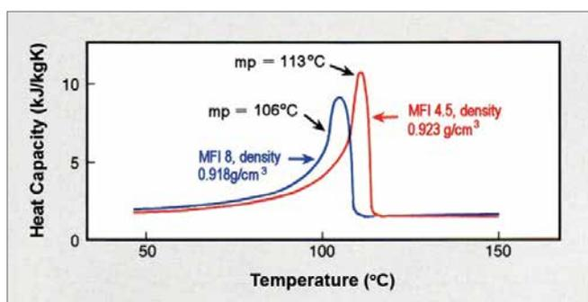
**Figure 15: Melting Point and Heat of Fusion for Alkathene LDPE Extrusion Coating Polymers. (Determined by Differential Scanning Calorimetry)**
