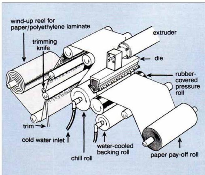
**Figure 2:** Typical Extrusion Coating Line for a Paper/Polyethylene Laminate
