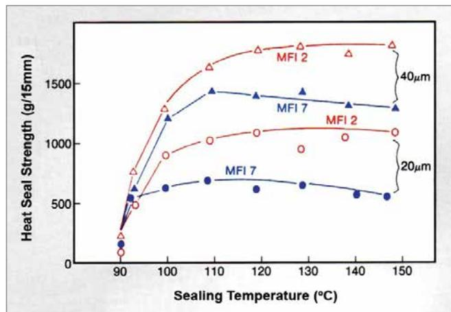
**Figure 16:** Relationship between MFI Values, Heat Seal Strength and Sealing Temperature
