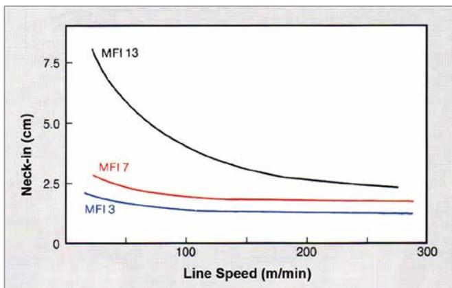
**Figure 6:** Effect of Line Speed on Neck-in for Several Alkathene LDPE Grades of Different MFI
