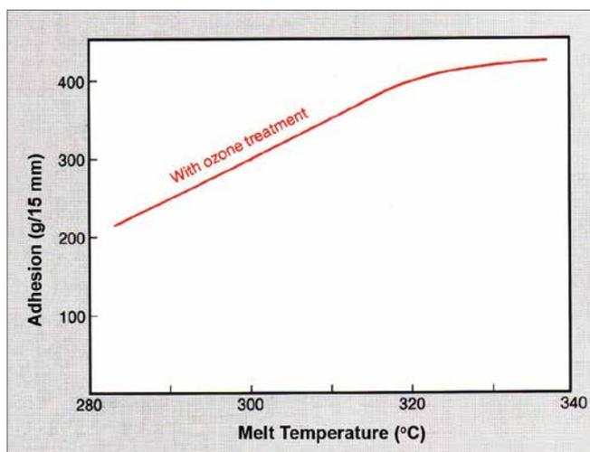
**Figure 9:** Effect of Melt Temperature and Ozone Treatment on Adhesion of Extrusion-Coated LDPE to Aluminium Foil
