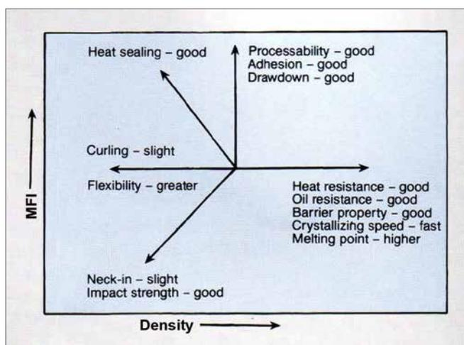
**Figure 1:** Influence of MFI and Density of Low Density Polyethylene on Processability and Laminate Properties
