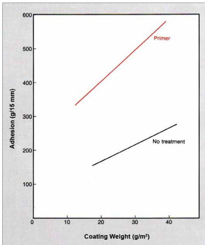
**Figure 13:** Typical Effect of Coating Weight on Adhesion of Extrusion-Coated LDPE to Aluminium Foil (60 m/min, 307°C)
