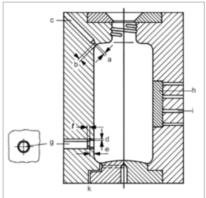
**Figure 35: Suitable Methods for Mould Cavity Venting**
