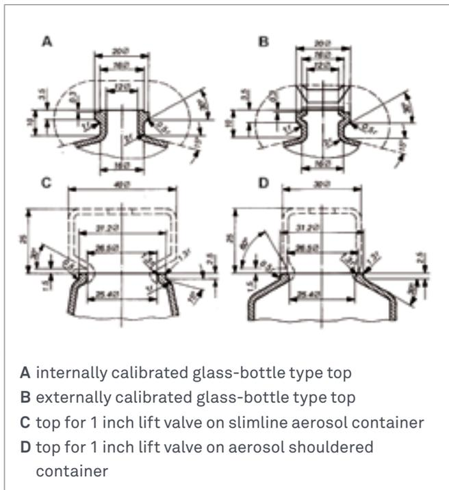
**Figure 44:** Design Recommendations for the Top of an Aerosol Container
