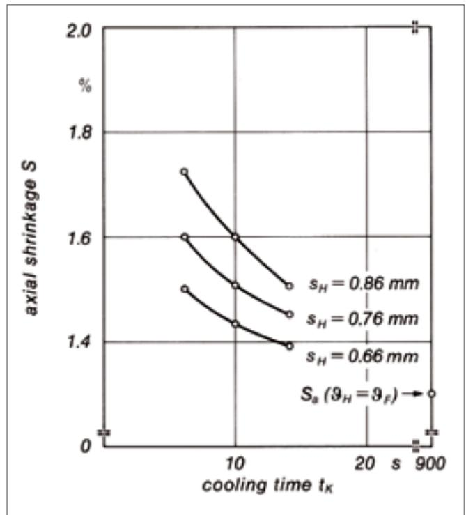
**Figure 37b:** Axial Shrinkage of Rotationally Symmetrical High Shouldered HDPE Bottles with Various Wall Thicknesses as a Function of Cooling Time in the Blow Mould Under Blowing Pressure with Compressed Air Convection Cooling Melt Temperature 190°C, Mould Temperature 14.5°C, Inflation Ratio 2.1 : 1, Blowing Pressure 0.9 MPa
