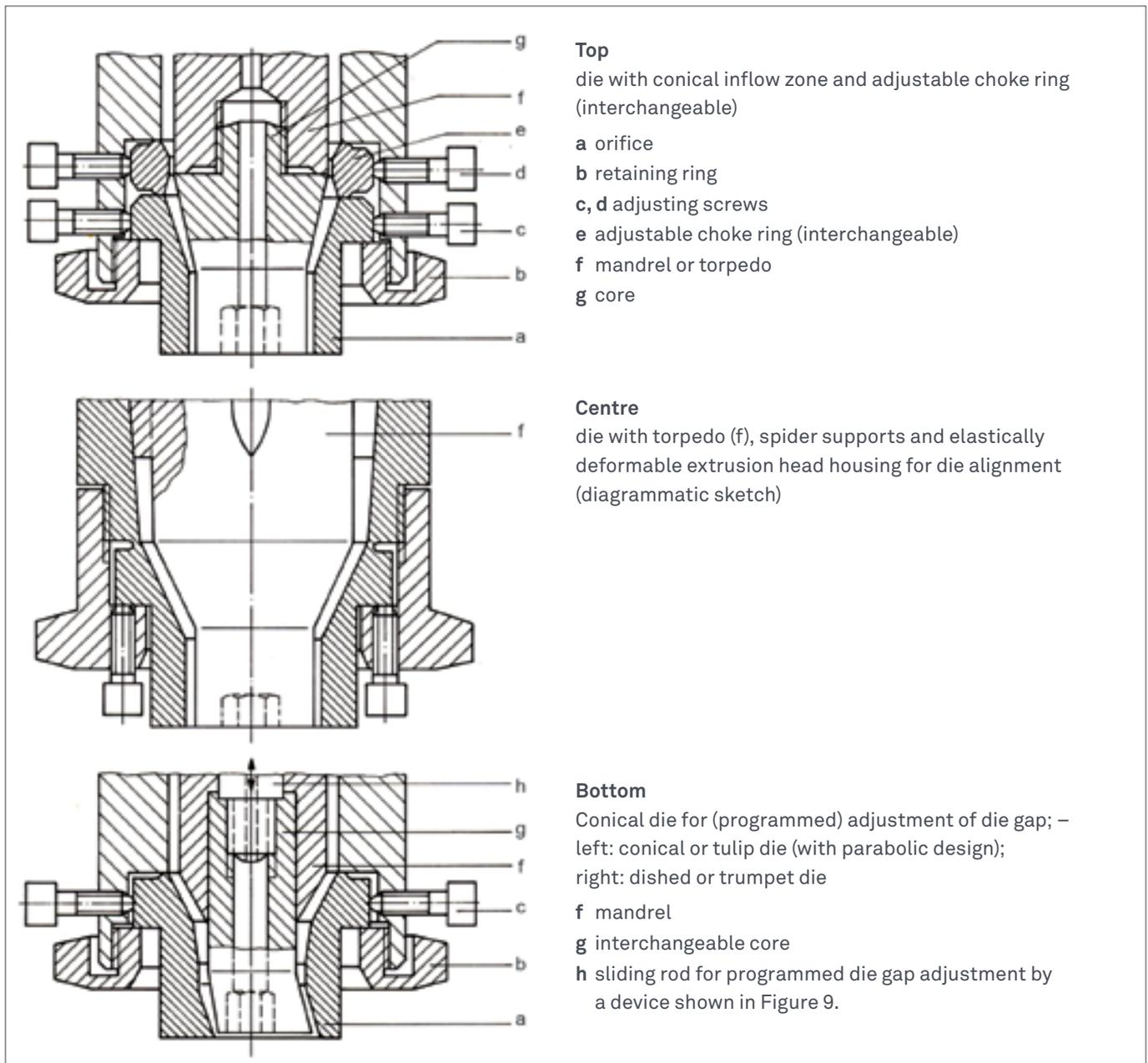
Figure 11: Conical Dies
