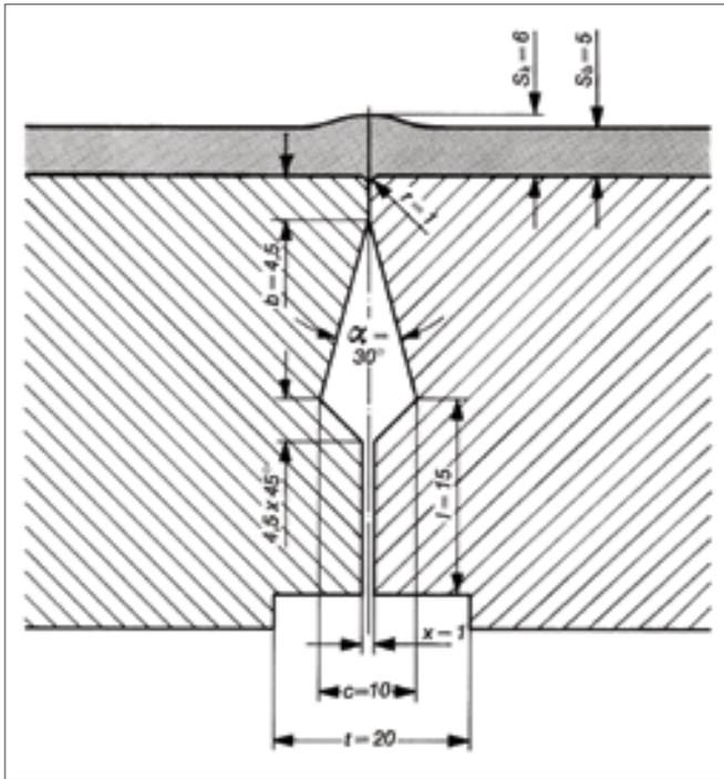
**Figure 33: Optimized Mould Base for a 60 L Can Made from HDPE**
