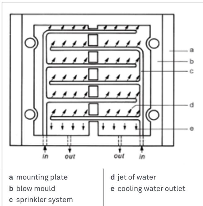
**Figure 28: Sprinkler (boundary layer) Cooling**
