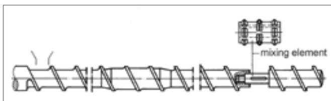
**Figure 1: Extruder Screw with Mixing Elements**
