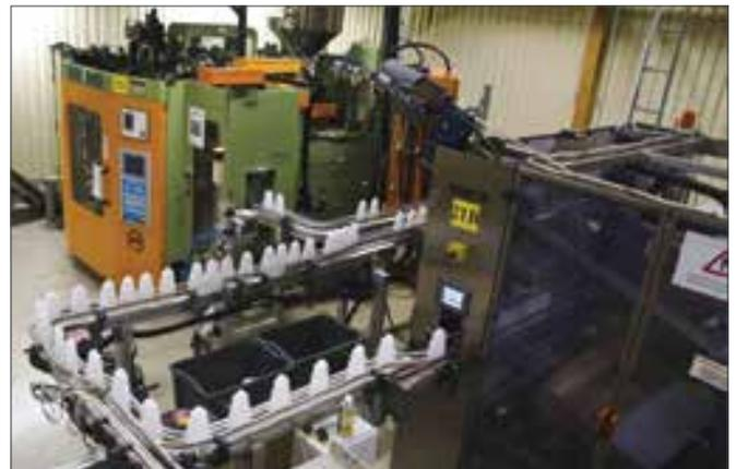
**Figure 5:** Dual Parison Blow Moulding Machine
