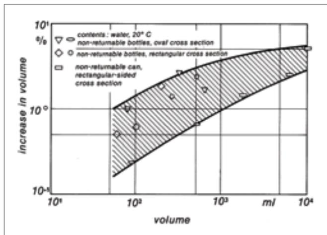
**Figure 45:** Increase in Volume of Non-returnable Bottles and Cans Made of HDPE Caused by Hydrostatic Pressure
