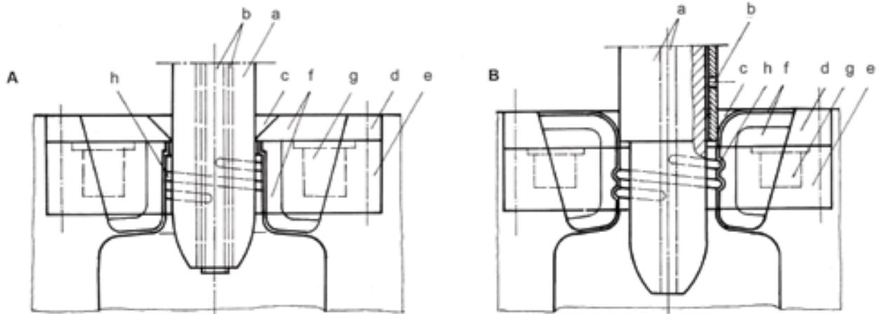
**A** Internal calibration of a bottle neck while blowing through the mandrel
