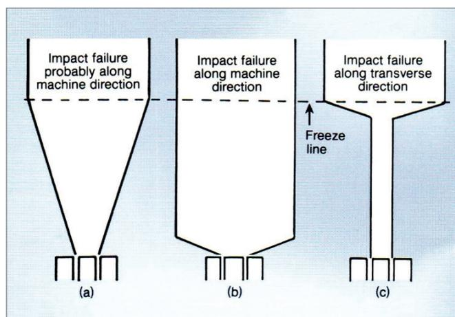
Figure 5: Hypothetical Modes of Drawing of a Film Bubble
