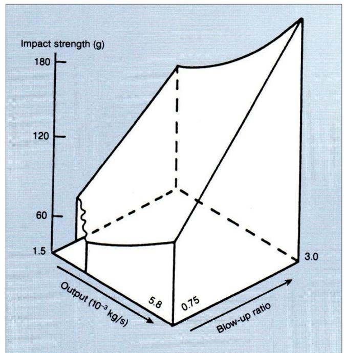
Figure 4: Variation of Impact Strength with Blow-up Ratio and Output Rate of an Alkathene LDPE Grade of MFI 2.0 and Density 0.921 g/cm<sup>3</sup> (Film Thickness 38 micron)
