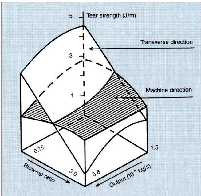
Figure 2: Variation of Tear Strength with Blow-up Ratio and Output Rate of an Alkathene LDPE Grade of MFI 2.0 and Density 0.921 g/cm<sup>3</sup> (Film Thickness 38 micron)
