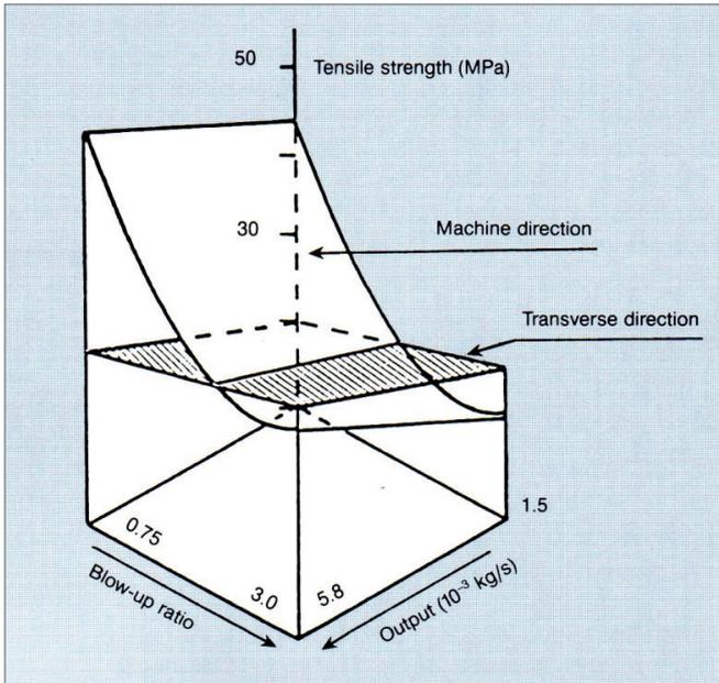
Figure 1: Variation of Tensile Strength with Blow-up Ratio and Output Rate of an Alkathene LDPE Grade of MFI 2.0 and Density 0.921 g/cm<sup>3</sup> (Film Thickness 38 micron)
