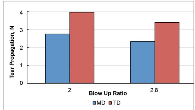
Figure 3: Effect of Blow-up Ratio on Tear Propagation for Alkamax mLLDPE Grade of MFI 1.0, Density 0.918 g/cm<sup>3</sup> (Film Thickness 25 micron)
